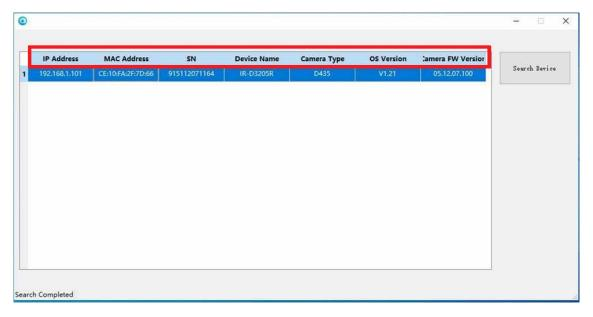
**IP Address :** The network IP is automatically assigned. You can disable the "DHCP" to change the IP Address.
