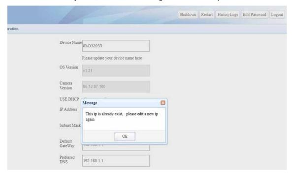
**Step 5** Enter the new IP, and click "update config". When the progress bar shows100%, the IP address changed successful, then the device will be restart.
